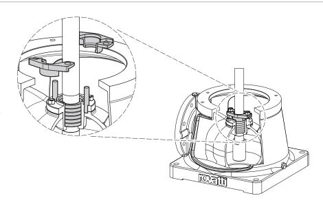
The V series vertical lineshaft pumps are designed to operate also with water level fluctuations and submerged impellers allot the pump di be started without need of priming.
